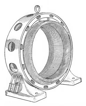
FIG. 137. Primary core and windings of a. c. induction motor.
